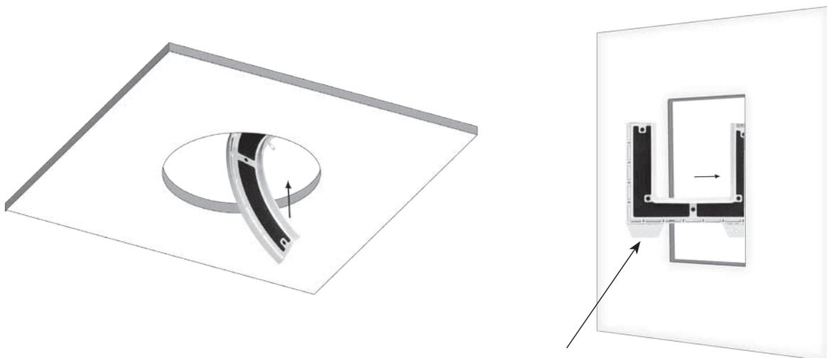
**Note:** Break off all four mounting tabs before installing horizontally to avoid interference with the wall studs.
